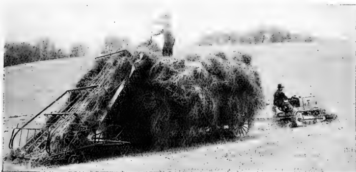
FIG. 243.—A caterpillar tractor drawing a wagon and hay loader. (Cleveland Tractor Co.)
